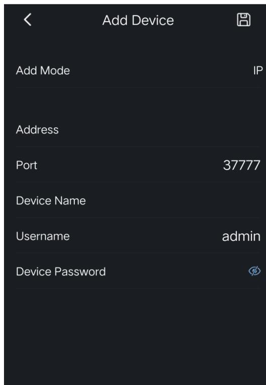
**Step 3** Enter Address (IP address of the VTO), Device Name, and Device Password.
